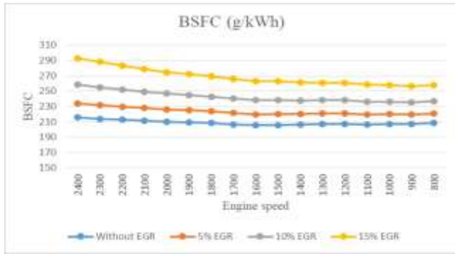
Graph 5: BSFC values at various engine speed for different EGR rates
