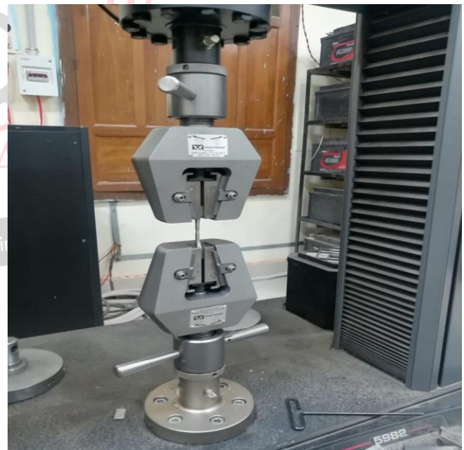
Figure: 2. Loading arrangement of specimen on Universal tensile testing machine.
