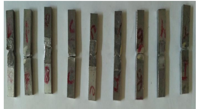
Fig-15 Specimens after Testing (Impact)
