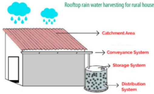
Figure 8 – Roof top rain harvesting of the building
