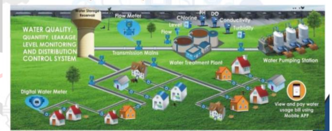
Figure 11 – Smart water management system
