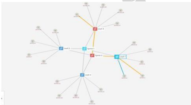
Figure 10, packet path after Add host intent from gui .
