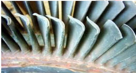
Fig 3: Fatigue Creep Failure
