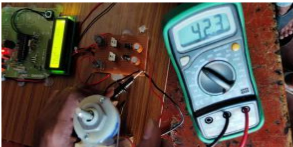
Figure11: Output voltage for pulse width 125 microseconds
