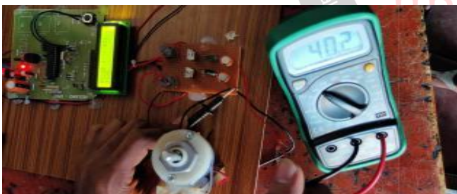
Figure 12: Output voltage for pulse width 199 microseconds
