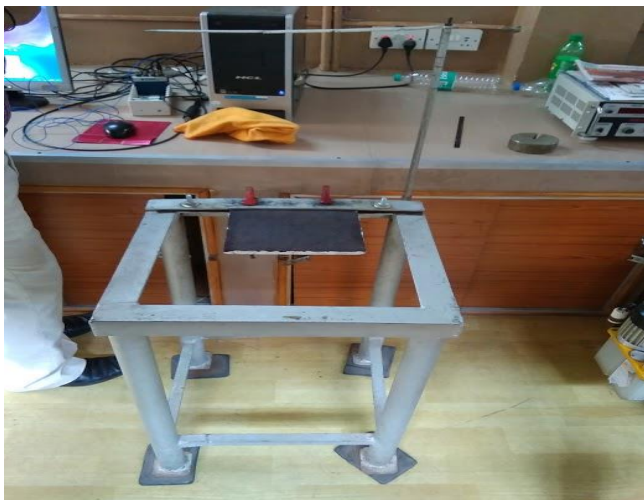
Figure 2.1. Loading arrangement of specimen for vibration damping modal analysis test
