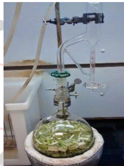
Fig. 2:- A Hydodistillation Clevenger type apparatus used to extract the Essential oils of O. sanctum and O. basilicum
