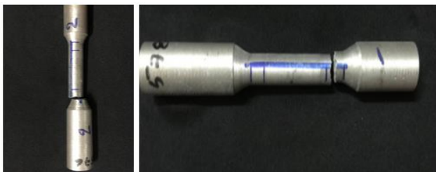
Figure 4 Tensile test break specimen
