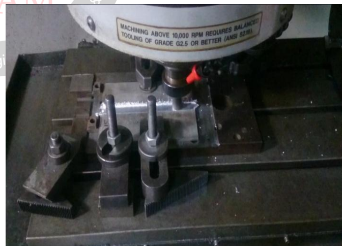
Fig. 4: Attachment of Fixture and plate on Machine
