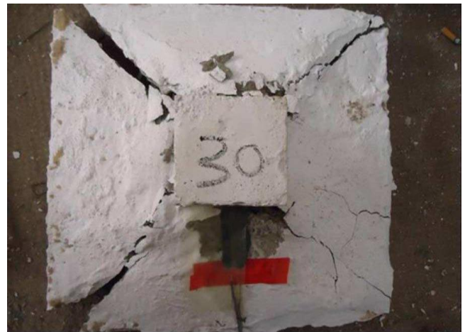
Fig. 4.2 Bottom Failure of 0 degree folded footing during a constant load
