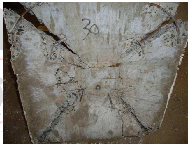
Fig. 4.4 Bottom Failure of 30 degree folded footing during a constant load
