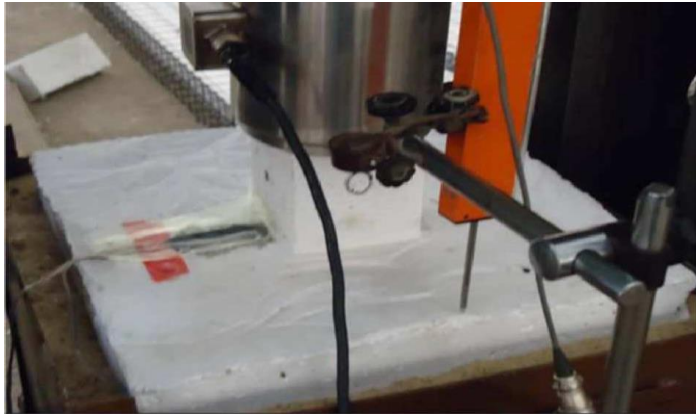
Fig 4.1 Calibrated loading in 0 degree footing
