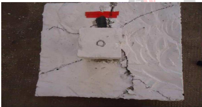
Fig. 4.4 Bottom Failure of 30 degree folded footing during a constant load
