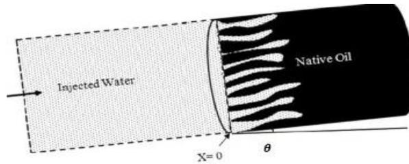
Fig. 1 Representation of instability phenomenon in a cylindrical piece of inclined homogeneous porous matrix
