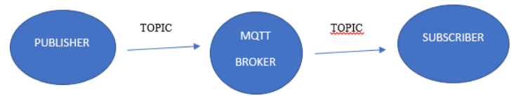
Figure 2: Simple MQTT protocol communication structure
