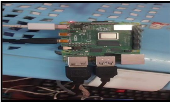
Figure 4: Connection of Raspberry Pi 4 to HDMI and USB Cables
