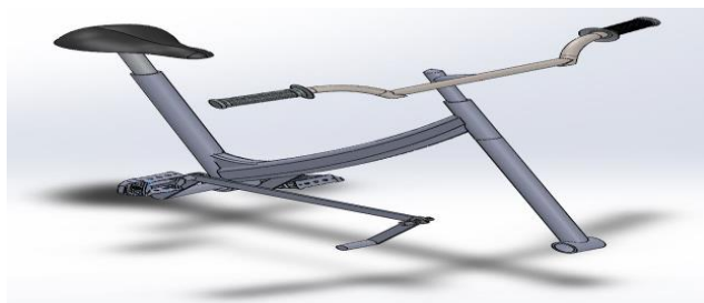
Figure 3: 4-bar Mechanism on bicycle pedal
