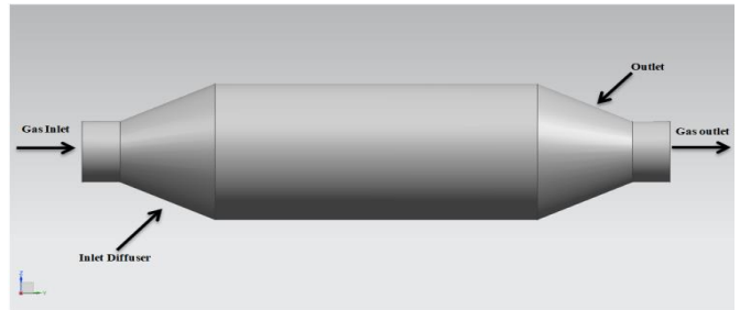
Fig.2 Schematic Structure of the Catalytic converter
