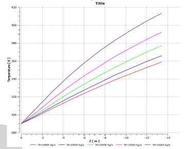
Plot 3 Temperature Distribution On the Corrugated Pipe at different Mass flows.
