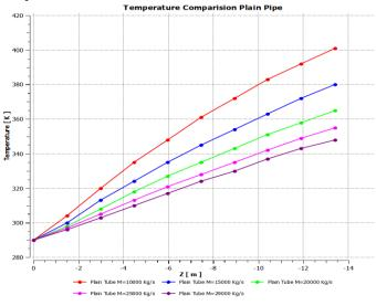
Plot 1 Temperature Distribution On the Plain Pipe at different Mass flows.
