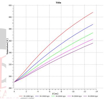
Plot 2 Temperature Distribution On the Semi Corrugated Pipe at different Mass flows.
