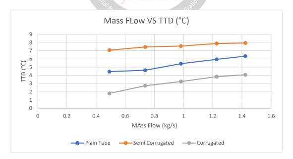
Plot 6 Mass Flow VS TTD for Different Pipes
