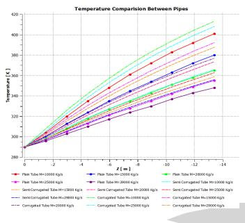
Plot 12 Temperature Distribution along the Length of the Pipe for Different Pipes.
