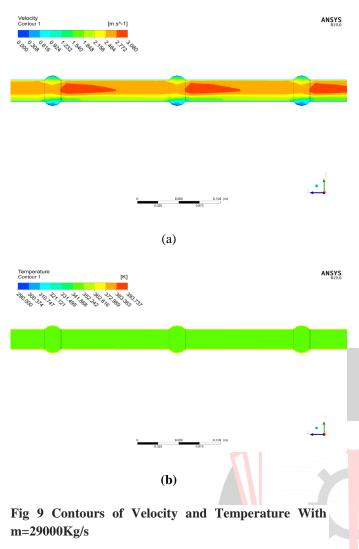
(a)Velocity Distribution in the Corrugated Pipe (b) Temperature Distribution of the Corrugated Pipe The Above Figures represents the Velocity and Temperature distribution of the water inside a Corrugated Pipe Where the Red Coloured region indicates high Velocity or the temperature from the figures The Velocity of the water in the single pipe with mass of 29000 Kg/s is 3.080 m/s after heat transfer in a steady state and the Exit cold water temperature 359.6895K.
