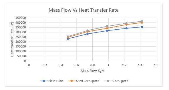
Plot 4 Mass flow Vs Heat transfer Rate in different Pipes
