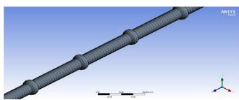
Fig 6 Meshing of the Corrugated Pipe.
