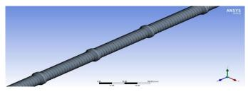
Fig 5 Meshing of the Semi Corrugated Pipe.
