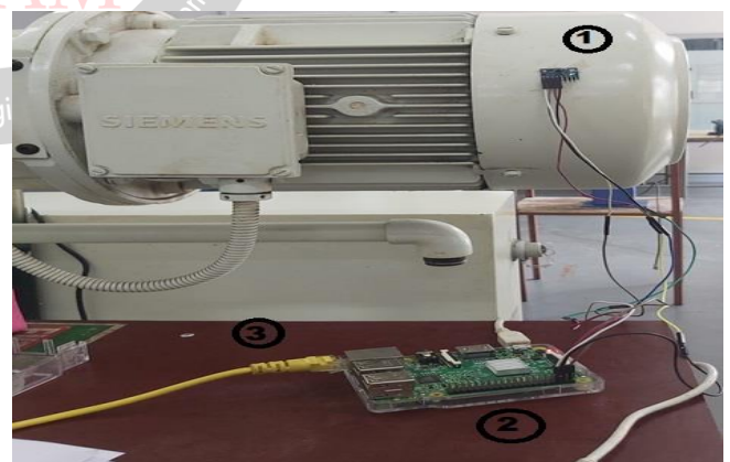
① GY-521 Board ② Raspberry-Pi 3 Model B ③ Ethernet cable
