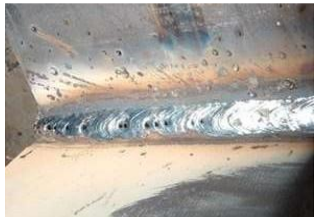
FIGURE 1 : POROSITY ON WELDMENT
