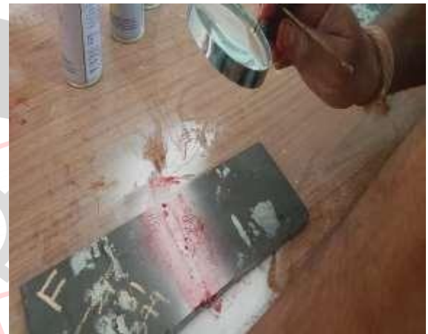
FIGURE 3: SPATTER ON FACE SIDE OF WELD
