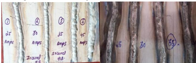
Fig 4.1 Bead on plate on Inconel 625 and Inconel 718.
