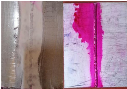
Fig 4.6 Liquid Penetrant Testing.
