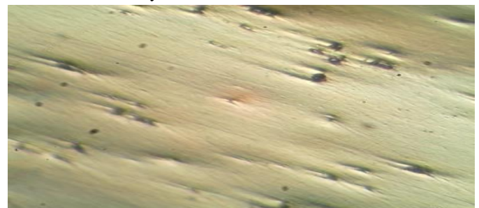
Fig 4.7 Micro structure of base metal Inconel 625.
