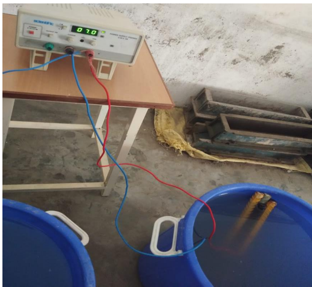
Fig.4 Accelerated Corrosion Process set up
