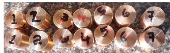
Figure 1.12 Hardness test specimens before test
