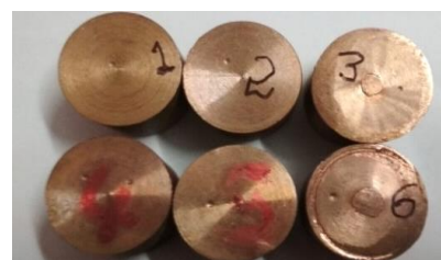
Figure 1.13 Hardness test specimens before test
