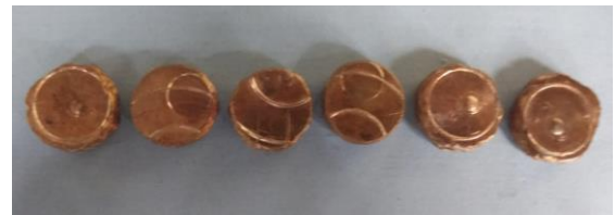
Figure 1.10 Compression Specimens after Test
