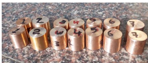
Figure. 1.9 Compression Specimens before Test
