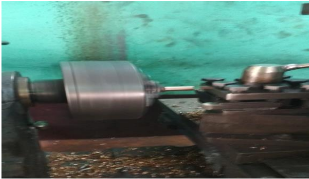
Figure:1.8 Machining of Casted Product
