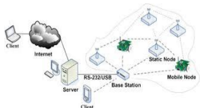
Fig. 1.1 : General structure of a static WSN
