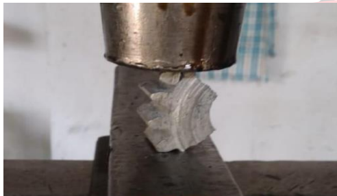
Fig.3 Testing of tangential load arrangement of gear
