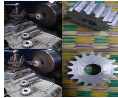
Fig. 1 Photographic view of fabrication of composite gears
