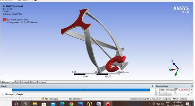
Fig 4.6 Applying torsional moment to the model.
