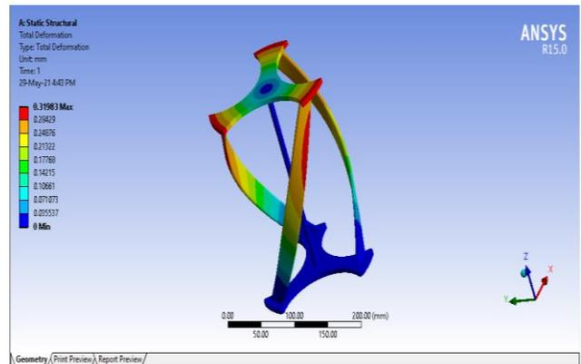
Fig 5.12 Total Deformation development in VAWT of 240mm height -Model-6
