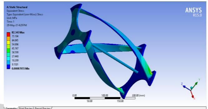
Fig 5.3 Equivalent Von-mises Stress Distribution in VAWT with 26mm Blade width-Model-2
