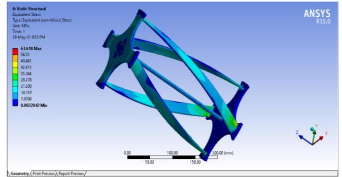
Fig 5.17 Equivalent Von-mises Stress Distribution in VAWT with 4 blades-Model-9
