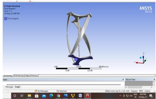
Fig 4.2 Applying fixed constraints in Ansys 15.0
