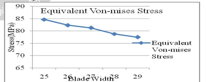
Fig 5.19 Effect of blade width on stress intensity
