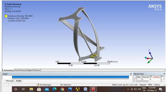
Fig 4.3 Applying rotational speed to the model in Ansys 15.0
