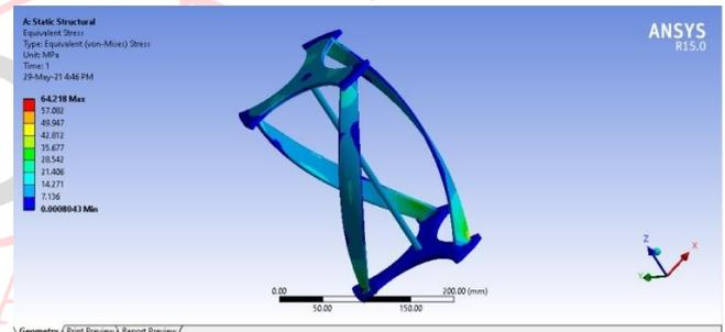
Fig 5.13 Equivalent Von-mises Stress Distribution in VAWT of 260mm height-Model-7
