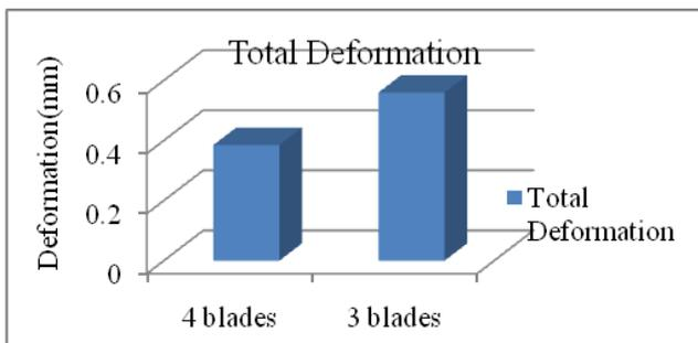
Fig 5.24 Comparison of deformation in 3 and 4 blades turbine
