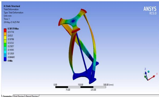
Fig 5.6 Total Deformation development in VAWT with 27mm Blade width-Model-3
