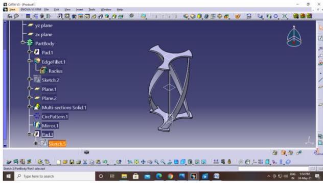
Fig 3.2 Final model of VAWT with 3 blades created in catia V5
