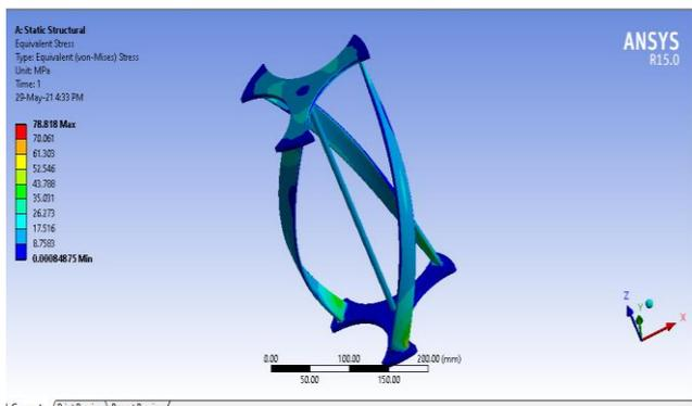
Fig 5.7 Equivalent Von-mises Stress Distribution in VAWT with 28mm Blade width-Model-4
