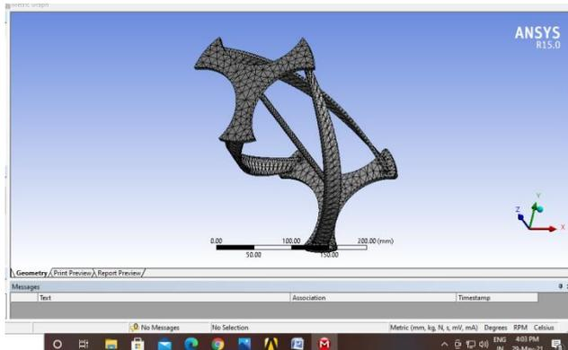
Fig 4.1 Meshed model of VAWT in Ansys 15.0
