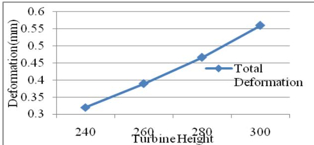
Fig 5.22 Effect of the turbine height on the deformation
