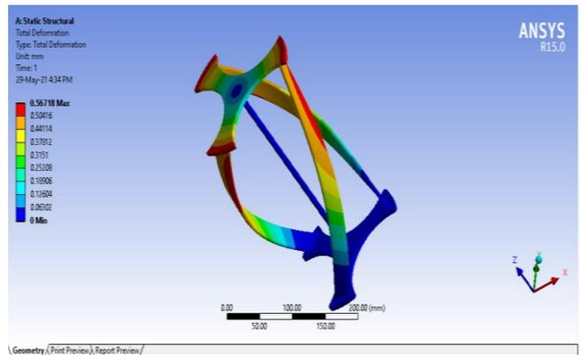
Fig 5.8 Total Deformation development in VAWT with 28mm Blade width-Model-4
