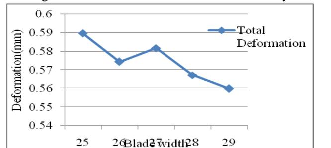
Fig 5.20 Effect of blade width on the deformation development
