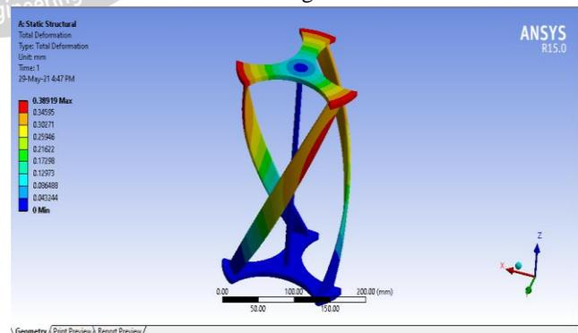
Fig 5.14 Total Deformation development in VAWT of 260mm height -Model-7
