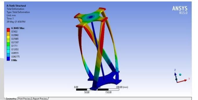
Fig 5.18 Total deformation development in VAWT with 4 blades-Model-9
