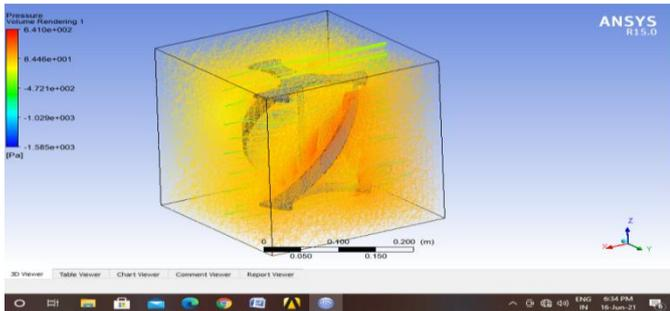
Fig 5.28 Pressure counter along the considered volume in fluid flow (CFX) analysis in Ansys 15.0
