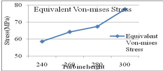
Fig 5.21 Effect of the turbine height on the maximum stress development
