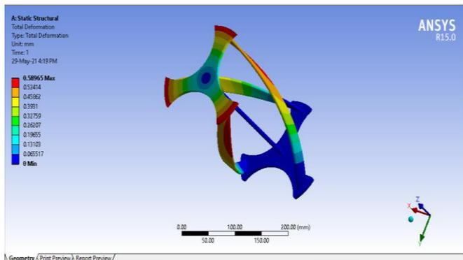
Fig 5.2 Total Deformation development in VAWT with 25mm Blade width-Model-1
