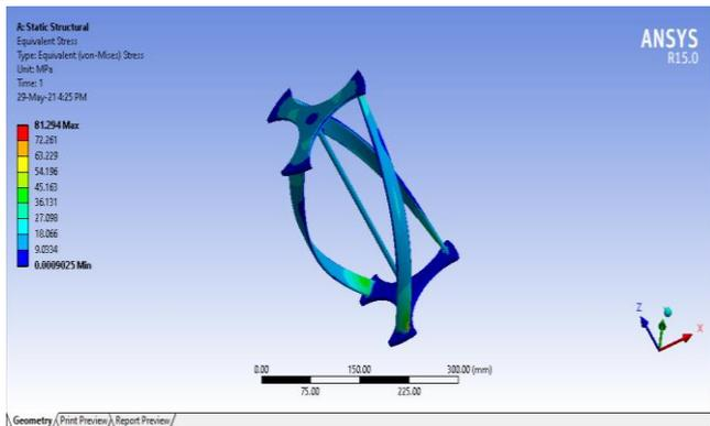
Fig 5.5 Equivalent Von-mises Stress Distribution in VAWT with 27mm Blade width-Model-3
