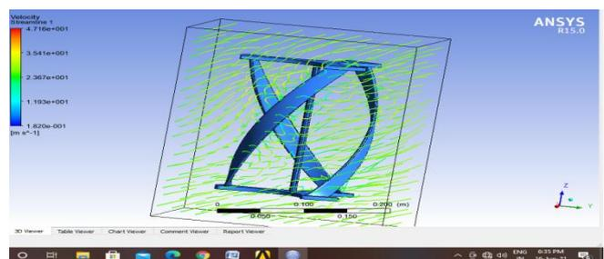
Fig 5.27 Velocity stream lines along the considered volume in fluid flow (CFX) analysis in Ansys 15.0
