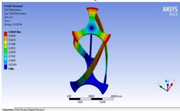
Fig 5.16 Total Deformation development in VAWT of 280mm height -Model-8
