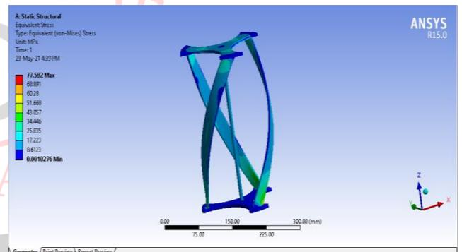
Fig 5.9 Equivalent Von-mises Stress Distribution in VAWT with 29mm Blade width-Model-5
