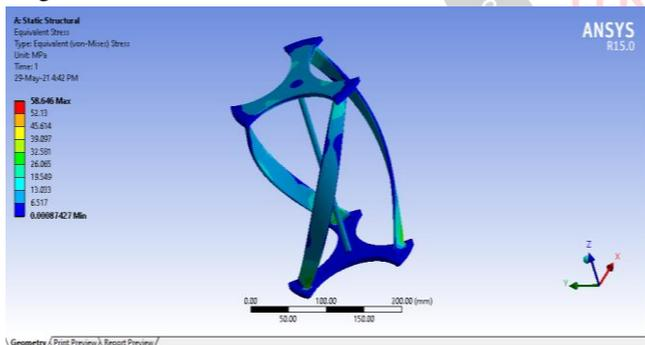
Fig 5.11 Equivalent Von-mises Stress Distribution in VAWT of 240mm height-Model-6
