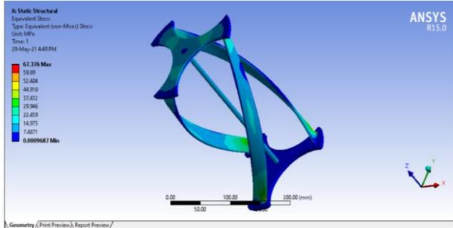
Fig 5.15 Equivalent Von-mises Stress Distribution in VAWT of 280mm height-Model-8
