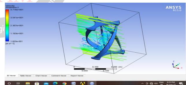
Fig 5.26 Velocity stream lines along mid plane (invisible) in fluid flow (CFX) analysis in Ansys 15.0
