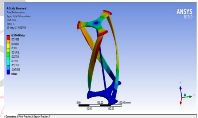
Fig 5.4 Total Deformation development in VAWT with 26mm Blade width-Model-2
