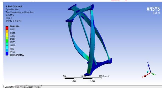
Fig 5.1 Equivalent Von-mises Stress Distribution in VAWT with 25mm Blade width-Model-1
