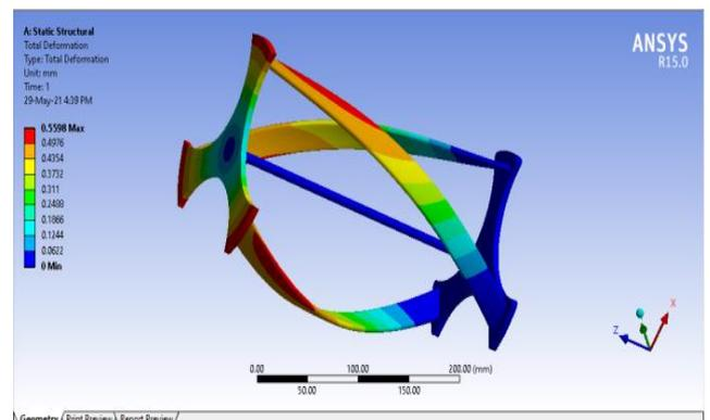
Fig 5.10 Total Deformation development in VAWT with 29mm Blade width-Model-5
