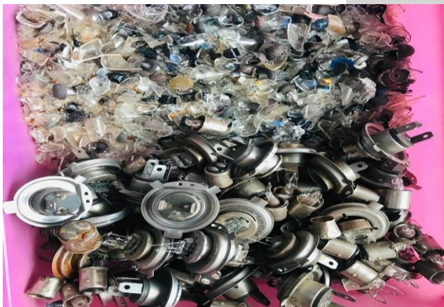
Figure 6- Crushed material of vehicular bulbs
