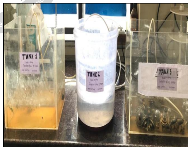
Figure 2- Aeration of bulb for cleaning in tank1, 2 & 3 respectively.
