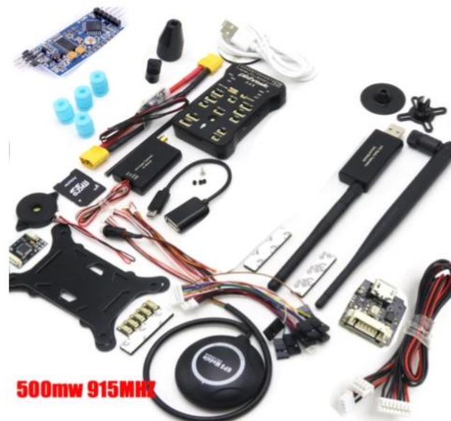
Fig.9. Pixhawk FCB with 915MHz telemetry, GPS, Shock Absorbing Plate
