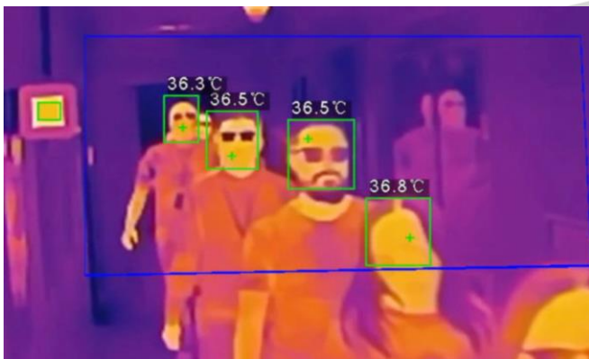
Fig[D] Thermal Temperature Detection
