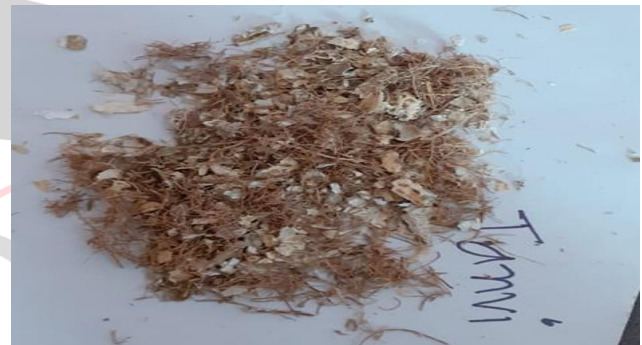
Fig. 1 Groundnut Shell and Coir Mixture
