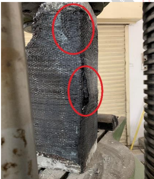
Figure no.3.10: Failure under uniform loading
