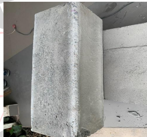
Figure no.3.7: column specimens with 5mm corner radii
