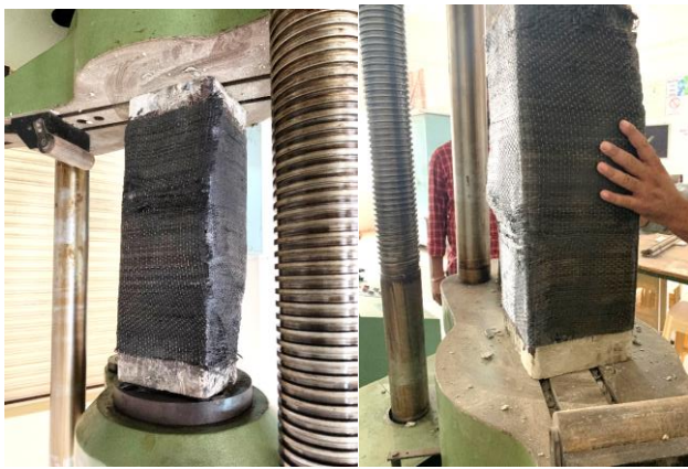
(a) (b) Figure no.3.9: Retrofitted column specimens under uniform loading
