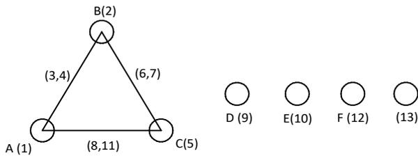
Figure 2. Linear graphs for  $L_{27}$  orthogonal array
