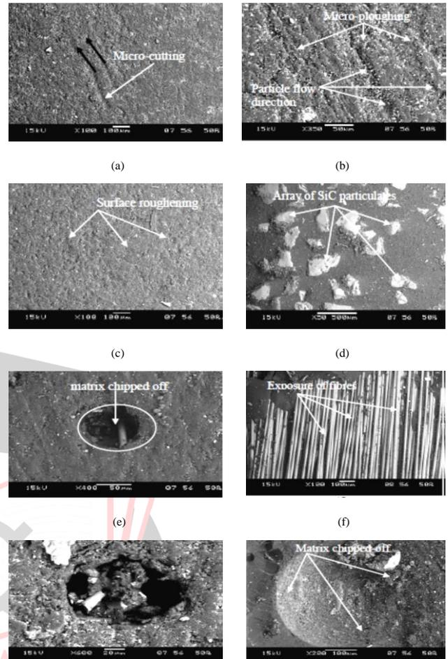
**Figure 10.** SEM micrographs of the eroded Glass-Vinylester composites filled with SiC.
