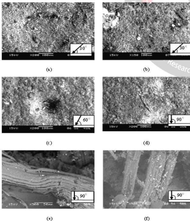
**Figure 9.** SEM images of eroded surfaces of Alumina filled PALF-Vinylester composites
