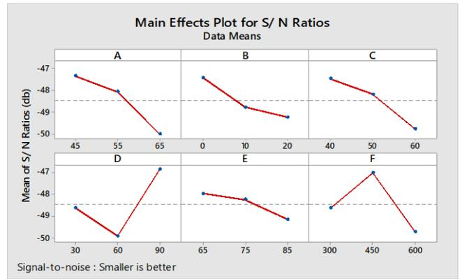
\*A= Impact Velocity, B=Filler content, C= Erodent Temperature, D=Impingement angle, E= Stand-off distance, F=Erodent Size
