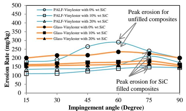
Figure 7. Effect of impingement angle on the erosion wear rate of SiC filled composites
