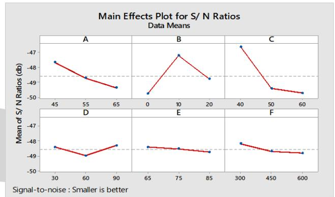
\*A= Impact Velocity, B=Filler content, C= Erodent Temperature, D=Impingement angle, E= Stand-off distance, F=Erodent Size
