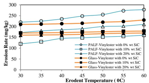
Figure 8. Effect of erodent temperature on the erosion wear rate of SiC filled composites
