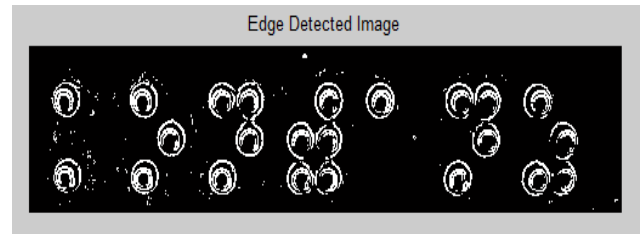
Figure-10: Edge detection by Sobel filter
