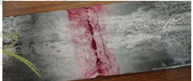
Inspection of weld on root side
