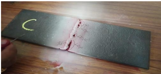
Defects on face side
