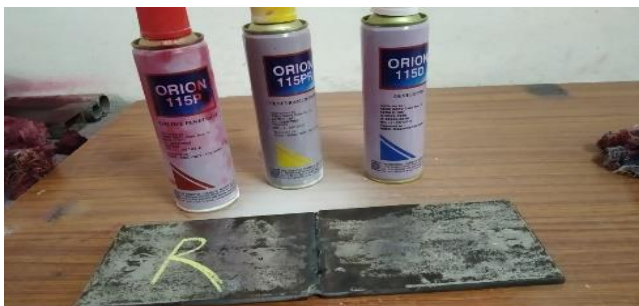
Dye penetratin on root side
