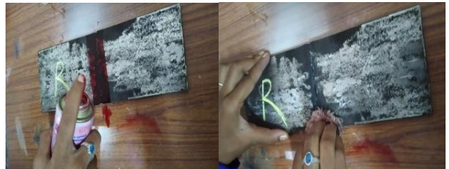
Application of penetrant on root side
