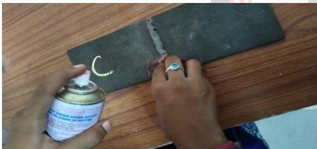
Post cleaning on face side
