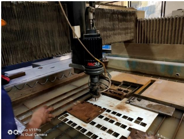
Figure 2. Working of AWJM
