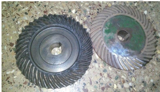
Fig.No.3.The image of Failure of Bevel gear
