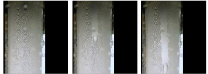
Fig. 5.1 Drop condensation on the inner surface of the tube.
