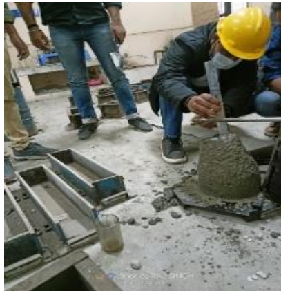
Fig. no. 5 Slump Value measurement
