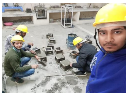
Fig. no. 7 Cube casting
