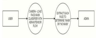
**FIG 2**: Firstly the user uses the camera present in the system to capture the image and make the classifier ready. Then the required classifier is loaded .Next the image of the face is extracted to determine if the mask is present or not. Finally
