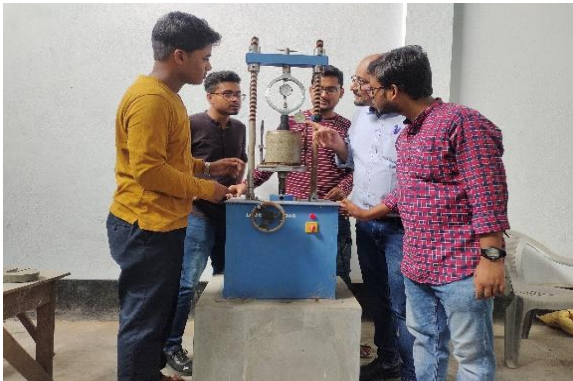
Figure 2 – California Bearing Ratio Test
