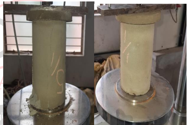
Fig.5.4: Failure pattern of fly ash based material specimen
