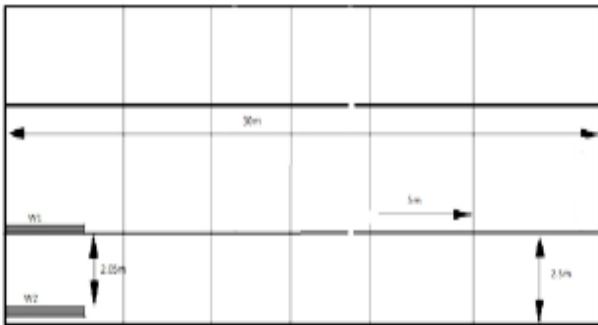
Fig.7: Position of IRC Class AA Tracked Load for Maximum Shear
