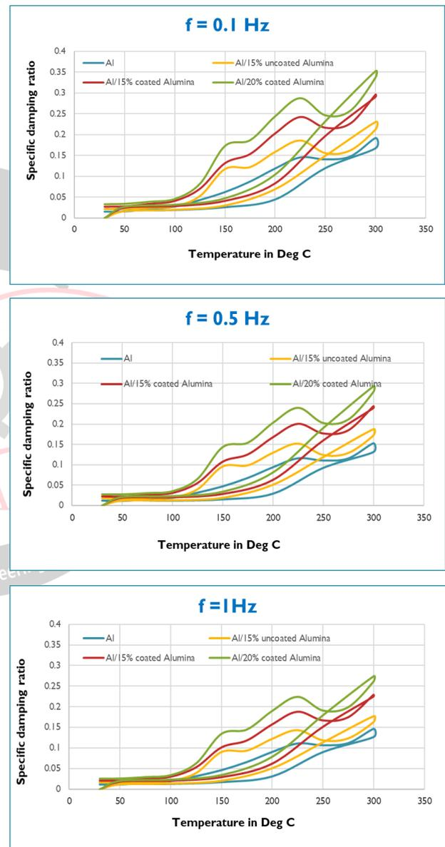
Fig. 1. Damping capacity ( $\tan \phi$ ) at a) 0.1 Hz b) 0.5 Hz and c) 1 Hz of Al alloy, Al/ uncoated Al<sub>2</sub>O<sub>3</sub> MMCs, and Al/ coated Al<sub>2</sub>O<sub>3</sub> MMCs as a function of heating and cooling at 10°C/min
