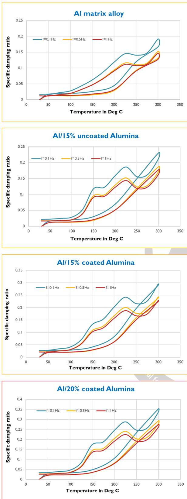
Fig. 2. Damping capacity ( $\tan \phi$ ) at a) Al matrix alloy, b) Al/ $\text{Al}_2\text{O}_3$  uncoated MMCs, and c) Al/ coated  $\text{Al}_2\text{O}_3$  MMCs for 0.1 Hz, 0.5 Hz, and 1 Hz of Al alloy, and as a function of heating and cooling at  $10^\circ\text{C}/\text{min}$
