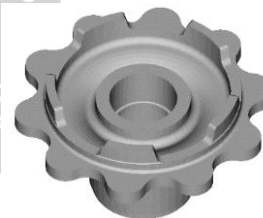
Fig-5: Importing the Model of the front hub into Autocast simulation software
