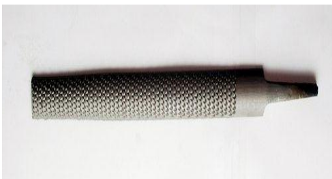
Fig -3: Half-Round wood rasp
