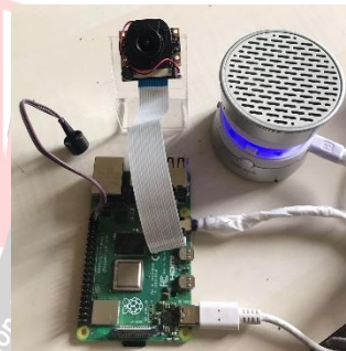
Figure 21: Drowsiness Detection System
