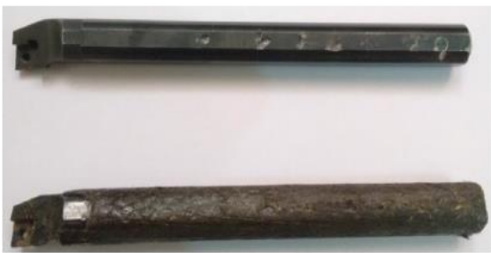
Fig.5.1 Photograph Standard and Laminated Boring Tool
