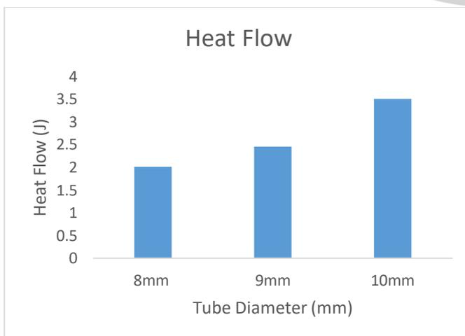
Figure 14: Heat flow vs tube diameter for R410 refrigerant
