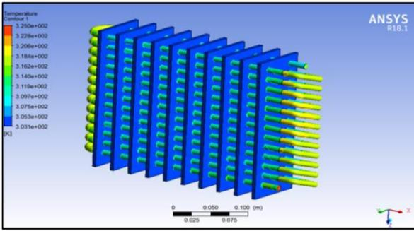
Figure 6: Temperature plot using R410 refrigerant and 8mm tube diameter
