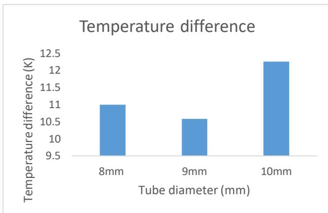
Figure 13: Temperature difference vs tube diameter for R410 refrigerant
