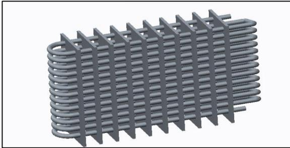
Figure 1: Condenser tubes assembled
