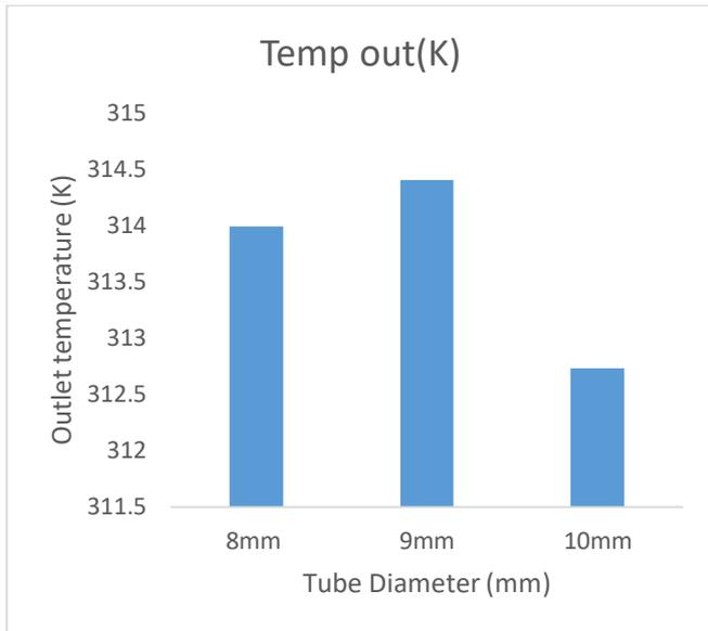
Figure 12: Outlet temperature vs tube diameter for R410 refrigerant
