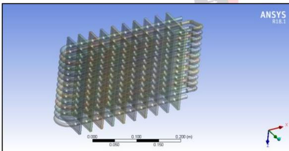
Figure 2: Imported CAD model in ANSYS
