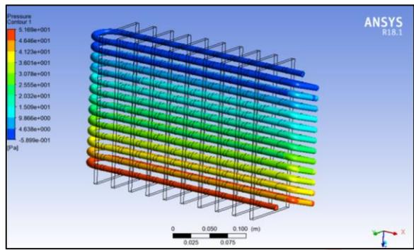
Figure 7: Pressure plot using R410 refrigerant and 8mm tube diameter
