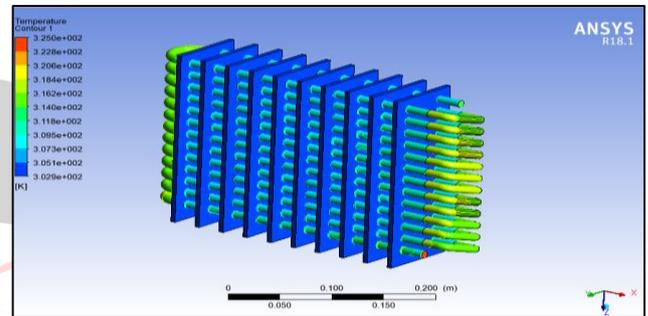
Figure 10: Temperature plot using R410 refrigerant and 10mm tube diameter
