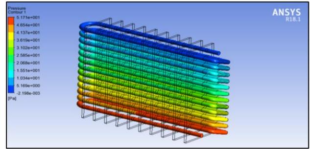
Figure 9: Pressure plot using R410 refrigerant and 9mm tube diameter
