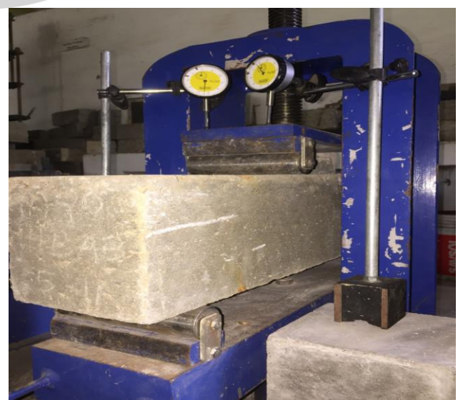
Fig. 1: Arrangement of Dial gauge with FTM
