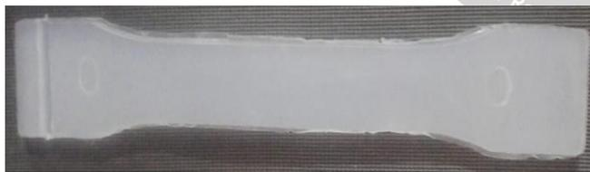
Fig. 1: Schematic diagram of the tensile test specimen (ASTM D638, Type-1)
